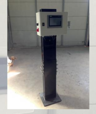
FCD-1100 allows to control the product flow used in each lube cycle. By using a flow meter at each spraying line, it is possible to find out the consumed lube quantity. Furthermore, FCD-1100 allows not only to view the consumed lube quantity but also to warn about a consumption failure by excess or shortage.
