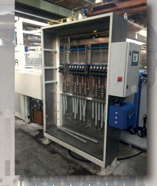
The management of each circuit will be or is performed through a hmi touchscreen where we can set different both flow and/or temperature warnings and /or alarms. The set point entered by the user allows the system to warn if the circuit value is beyond the work-range required.
