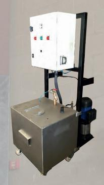
Whit SprayTank you have total control of the release agent that is provided to the lubricator.
